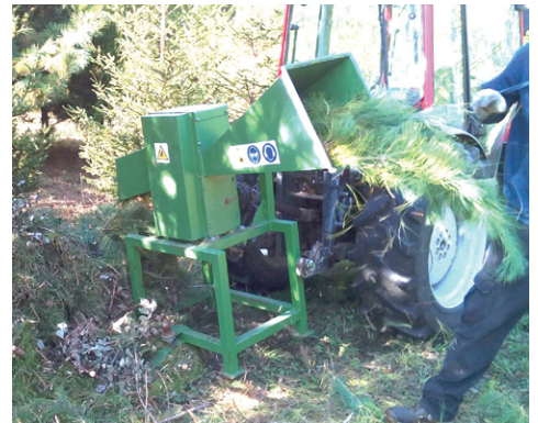
Figure 2.7: We can make wood chips from branches after tree pruning with the help of a shredding machine. Credit: Balázs Kulcsár
