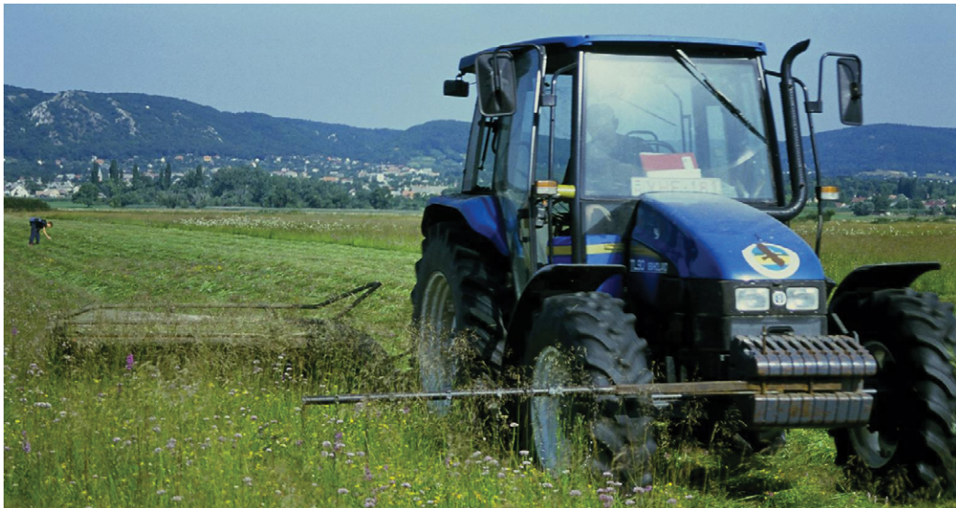
Figure 4.3: Flushing bar mounted on a tractor. Credit: Birdlife Hungary
