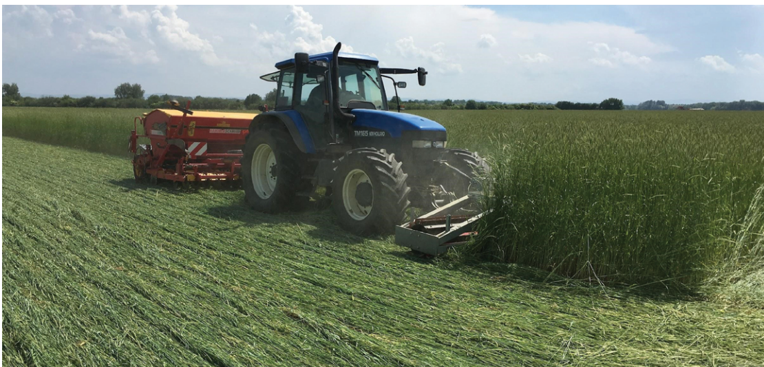
Figure 4.10: Field management in an agroecological way: Organic no-till with the roller-crimper method. Credit: GRAND FARM
