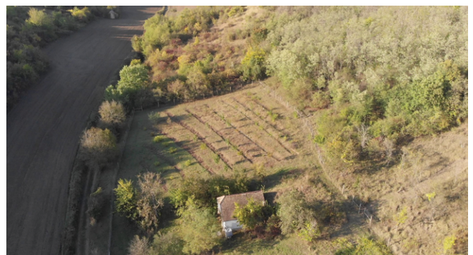
Figure 2.8: Swales on a steep site along contour lines. Credit: Etelka Kardos
