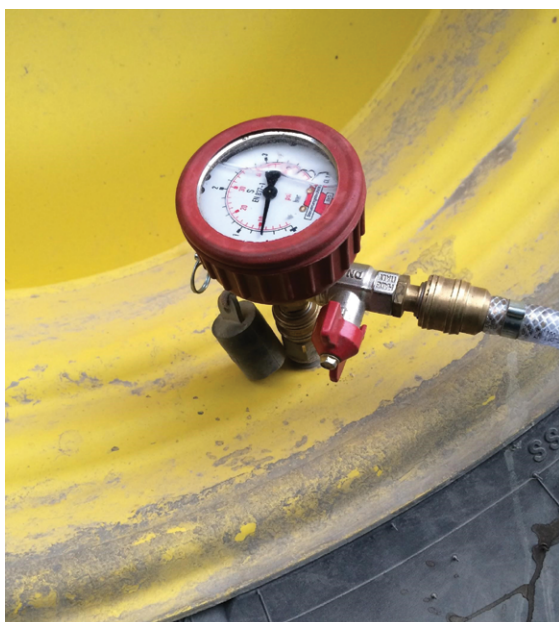
Figure 4.15: Simple tyre pressure adaptation system. Credit: GRAND FARM
