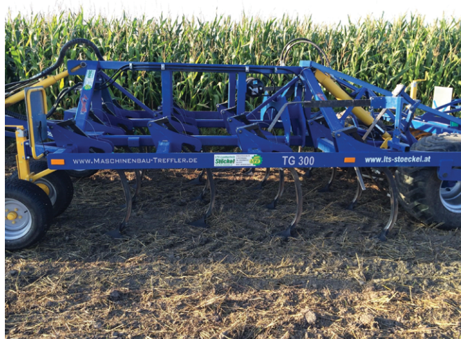
Figure 4.17: Example for specific equipment for reduced tillage (4 cm). Credit: GRAND FARM
